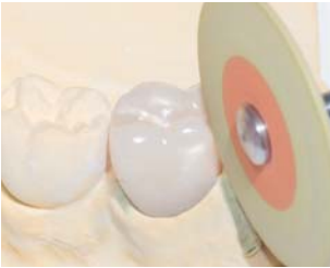
9770C: Mirror finish polishing of the external shape, Recommended rotary Speed: 7.000 – 12.000 rpm
